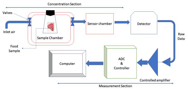
Fig 2.1: Schematic layout of a typical e-Nose Setup
