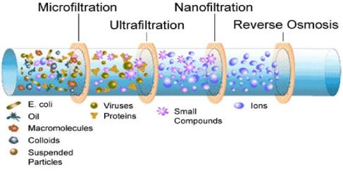
Fig.1 Different Membrane Separation
