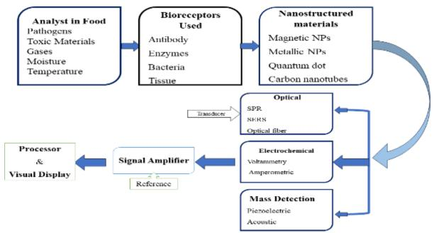
Fig. 1.1Schematic to illustrate the various nanosensors components
