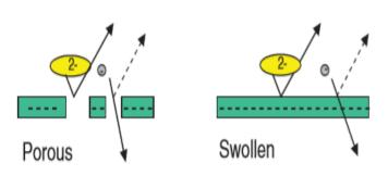
Fig. 3: Diagrammatic representation of the Donnan exclusion, porous and nonporous (swollen) NF membranes electrostatically repel charged species (such as ions) that bear the same electrical charge as the membrane material.
